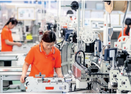
Employees at the wiring harness workshop of a private electronic enterprise in the Huayingshan Economic Development Zone of Huaying, southwest China's Sichuan province, perform harness crimping on an intelligent production line, April 18, 2025. (Photo/Qu Haiyang)
