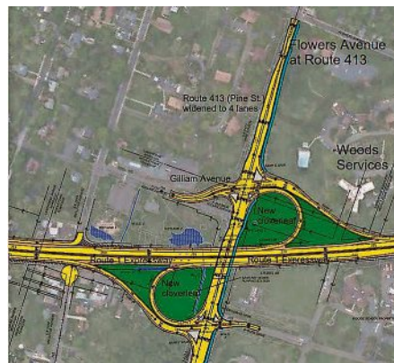
The Pennsylvania Department of Transportation's design would funnel Route 1 traffic at Route 413 into the circular sections of two new cloverleaves, with one connecting with southbound Route 413 toward Pennell, the other with northbound Route 413 toward Langhorne.
