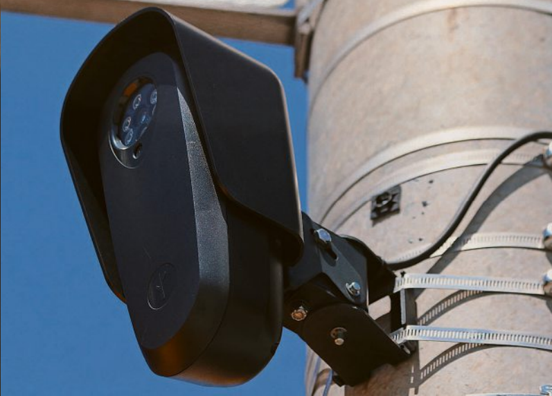
Flock cameras like this one on a utility pole in Pawtucket, Rhode Island, collect vehicles' license plate, make, model and color, information that is searchable by law enforcement agencies.
