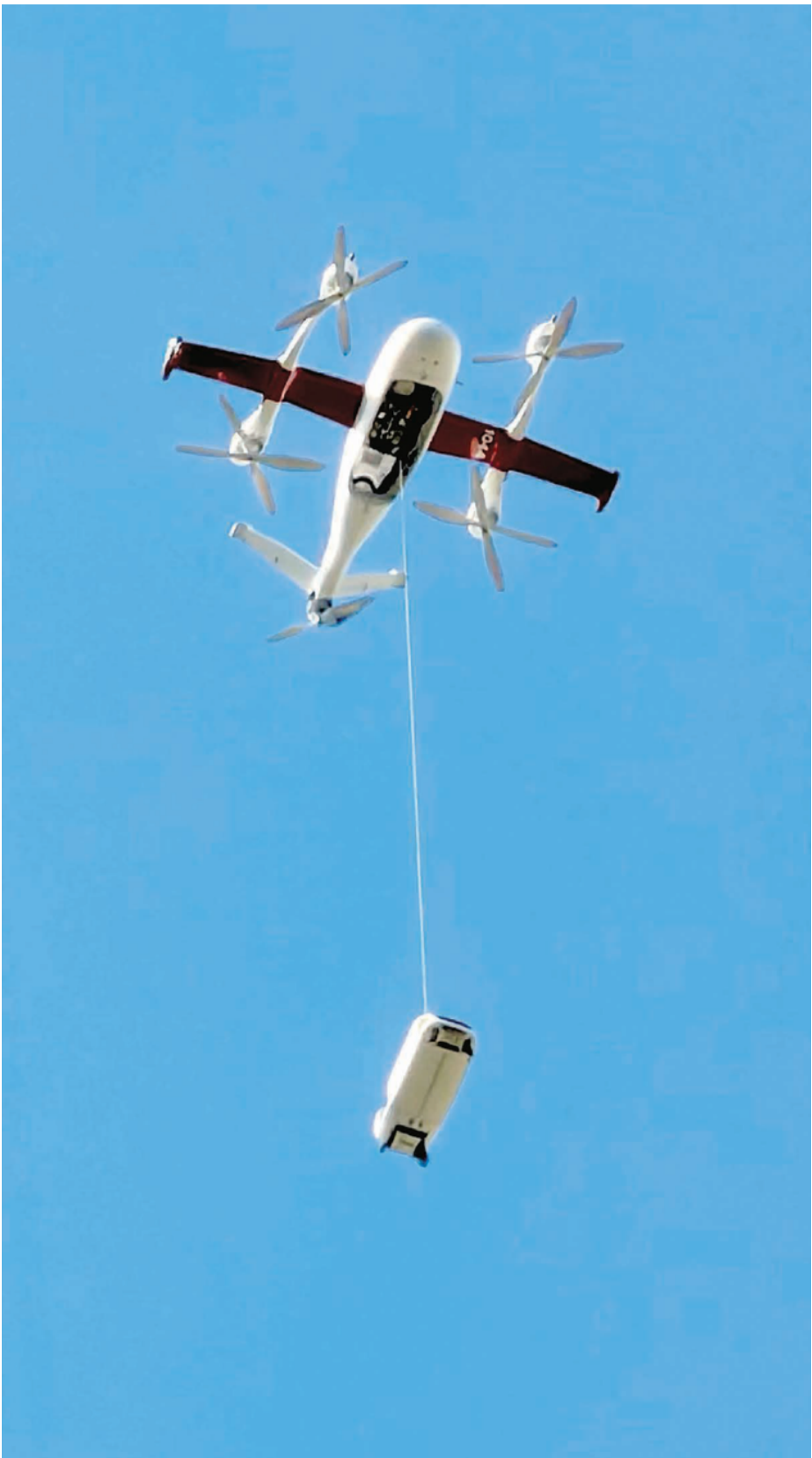
A Zipline drone lowers its delivery pod on a tether during a demonstration of Cleveland Clinic’s new prescription delivery service on Monday at its Beachwood Administrative Campus. The drone remains in the air while the pod descends to drop the payload. Ryan Cohick, cleveland.com
