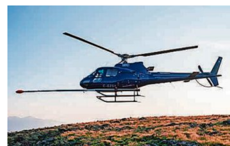
Geological survey flights will be conducted through fall 2026. A Eurocopter AStar-350 B3e helicopter is shown equipped with "stingers," an elongated sensor that collects data. PROVIDED BY USGS
