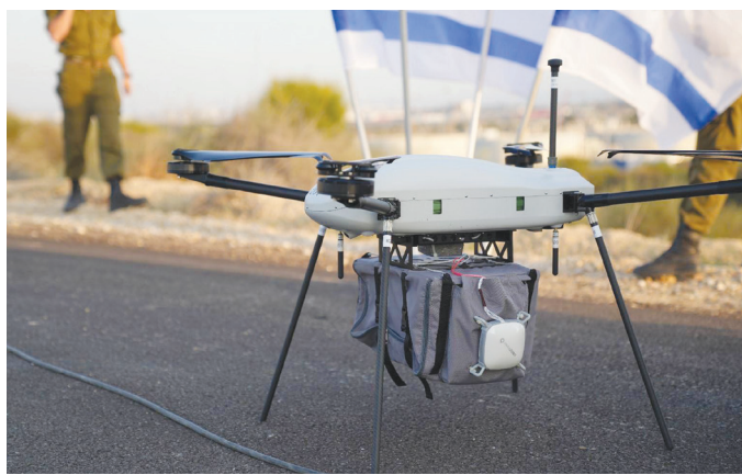
A DRONE developed by the IDF to deliver whole blood to the battlefield. (IDF)
