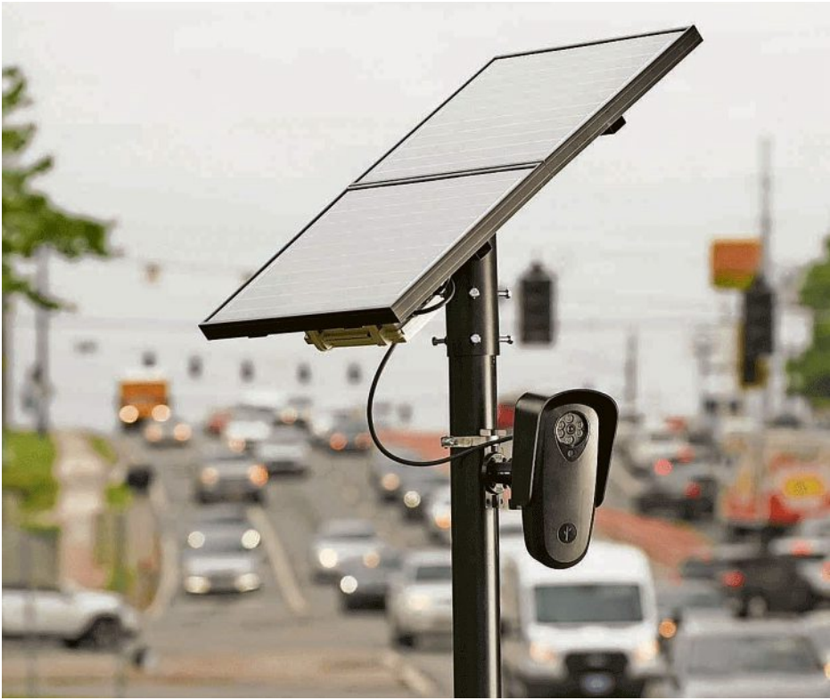
Flock Safety license plate-reading cameras are set up to scan all vehicles passing on a road. PROVIDED BY FLOCK SAFETY
