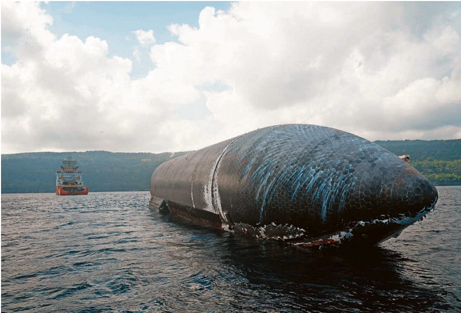
SpaceX last launched its Starship rocket July 24. The upper-stage, designated Ship 40, was able to slowly tip over and float in the ocean without exploding or sinking, as prior prototypes have done. PROVIDED BY SPACEX VIA REUTERS
