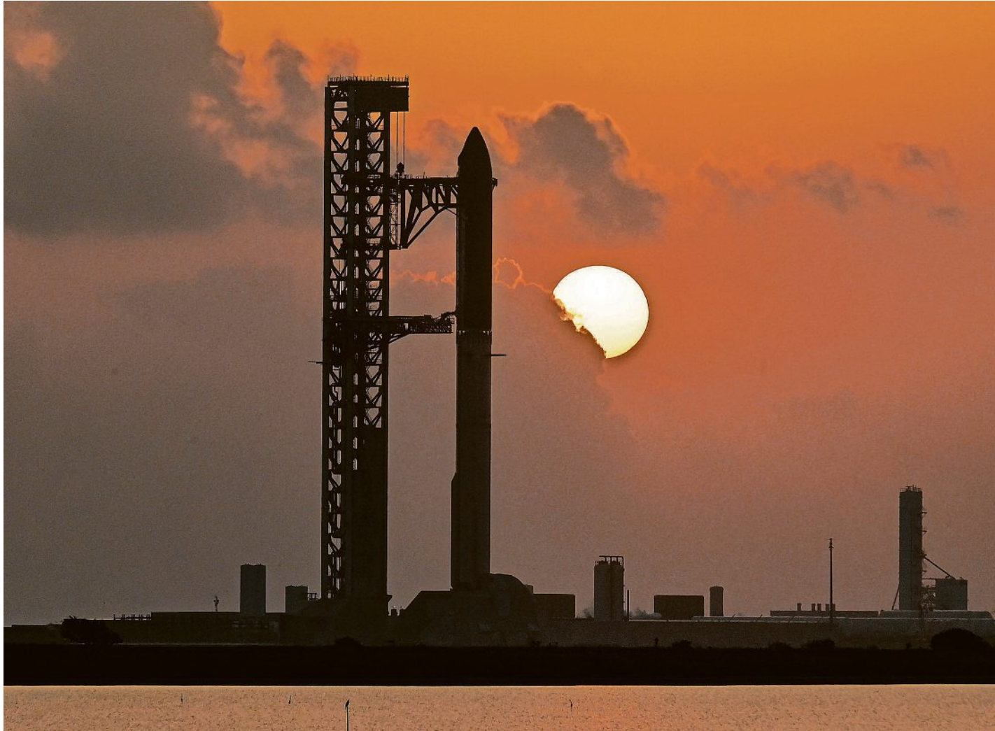
The fully integrated Starship spacecraft is composed of both a 236-foot-tall lower-stage booster known as Super Heavy and a 171-foot-tall upper stage simply called Starship. STEVE NESIUS/REUTERS
