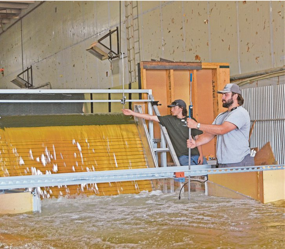
Each inch of water flowing through the model during a demonstration July 15 represents 2 feet of water in the actual reservoir following its planned expansion, said Chris Thornton, an associate professor and director of the hydraulics lab.
