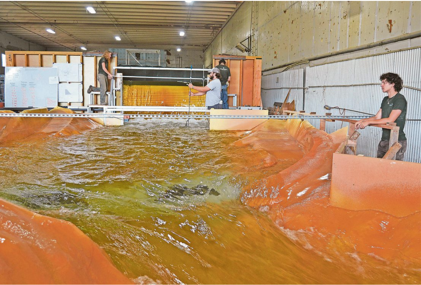
Students gather data using various instruments during a demonstration of maximum probable flood scenarios on a scale model of Halligan Reservoir's spillway and stilling basin on July 15 in a hydraulics laboratory at Colorado State University's Foothills Campus in Fort Collins. PHOTOS BY KELLY LYELL/THE COLORADOAN
