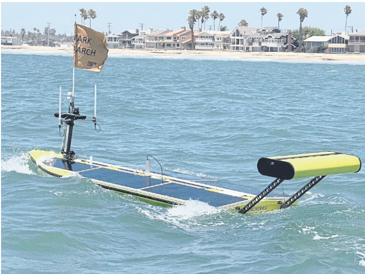
Cal State Long Beach Shark Lab researchers developed this robot watercraft that has acoustic receivers and cameras to listen and look for great white sharks. PHOTO BY CHRIS LOWE — CSULB SHARK LAB
